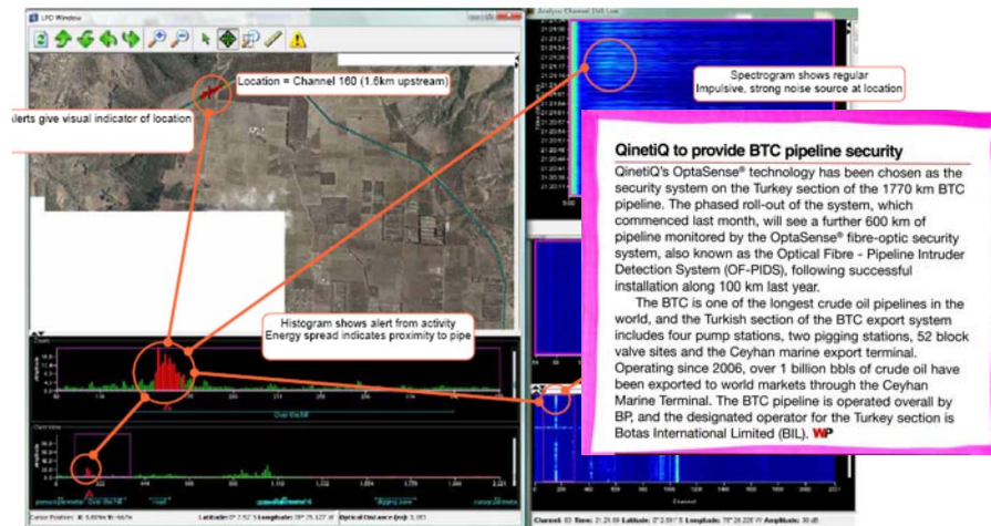
Figure 5: Example of manual digging activity on a pipeline deployment showing the graphical alerts as well as the more detailed analysis information revealing the nature of the threat. The digging was not a simulation but an actual threat event noted during deployment.
